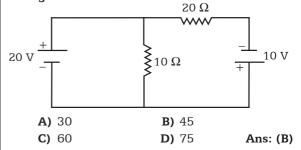
117. Determine the power dissipated (in W) by the  $\Omega$  resistor in the circuit given below.
