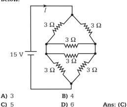
119. Determine the maximum power (in W) transferred from the source to the load of the circuit given below.
