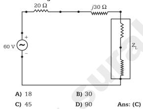
120. Determine the Norton's current (in A) and Norton's resistance (in  $\Omega$ ) respectively, for the given electrical circuit.
