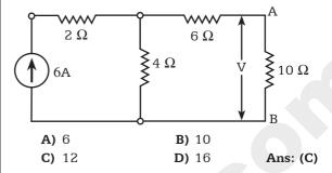
115. What will be the value of source impedance (in Ohms) for transmitting maximum power to the load in the circuit given below?
