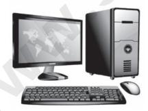
(i) Input unit: Input unit is used to feed any form of data to the computer, which can be stored in the memory unit for further processing. Example: keyboard, mouse etc.
